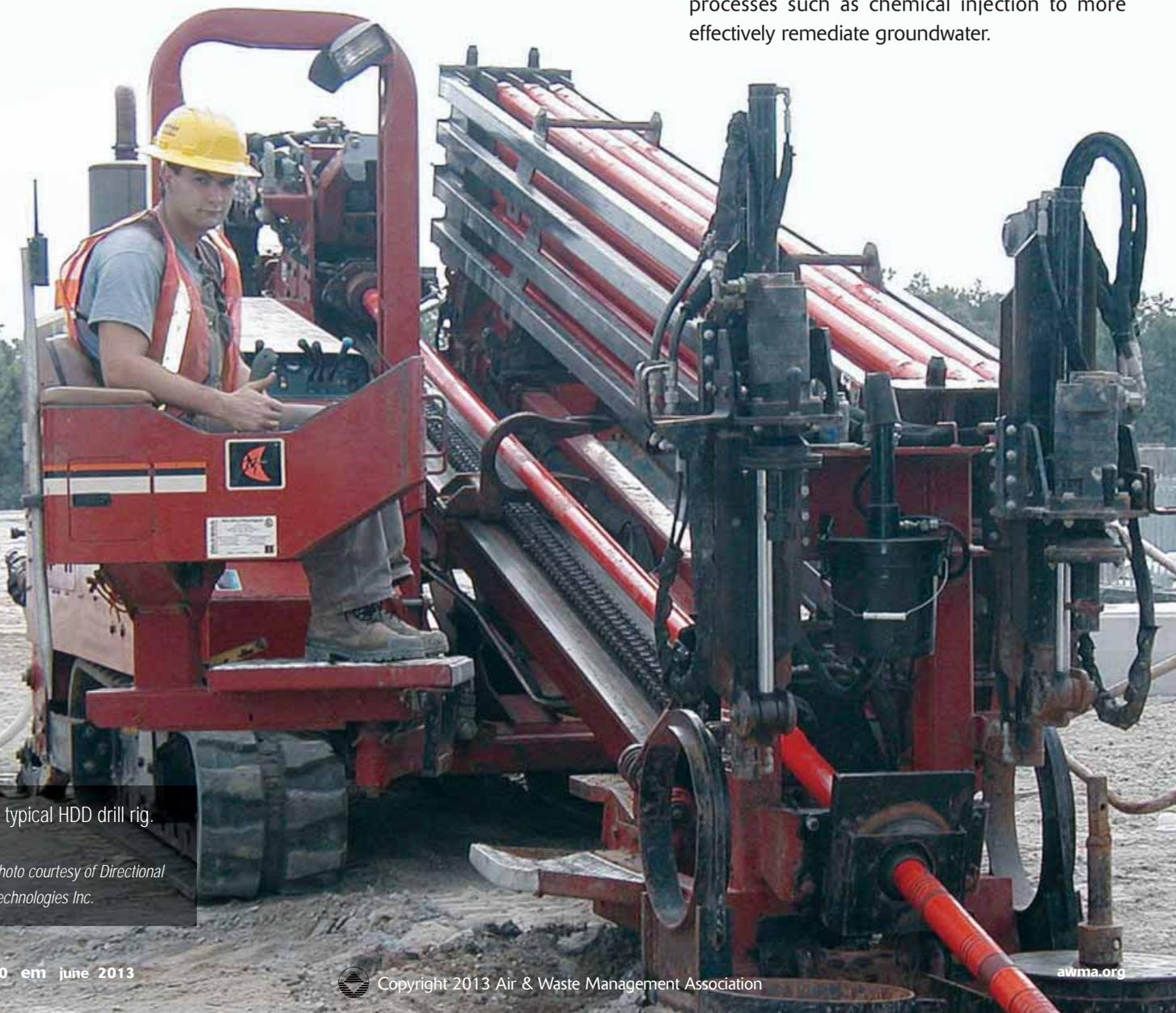
A typical HDD drill rig
