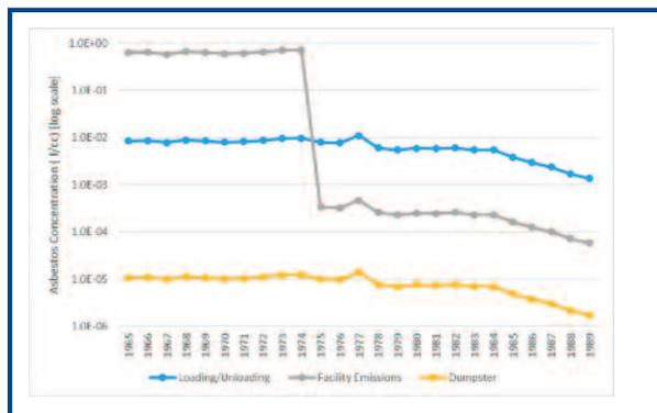
**Figure 3.** Annual average air concentration by source for receptors <500 m.
