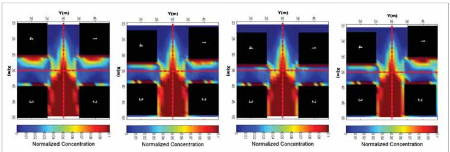
Figure 3. Four of the trade-off solutions for the 2x2 array problem. For the test problem, the wind is blowing from left to right and the normalized concentrations are shown at approximately the breathing height of a person.
