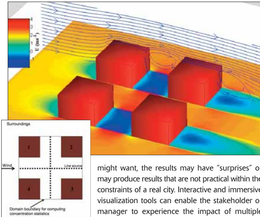
Figure 2. (inset) Schematic of the 2x2 building array problem. The buildings are labeled 1-4 and the pollution sources are shown as dashed lines between the buildings. Illustration of the 3D velocity field used to drive the pollution dispersion. Colored contours are velocity component in the mean wind direction.
